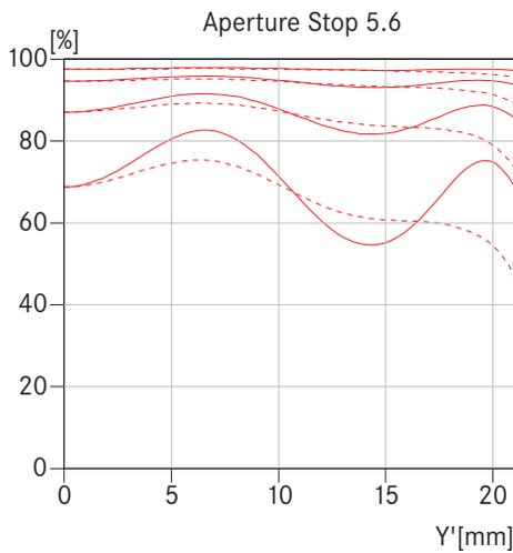
The MTF is indicated at full aperture, at f/2.8 and at f/5.6 at long taking distances (infinity). Shown is the contrast in percentage for 5, 10, 20 and 40 lp/mm across the height of the 35 mm film format, for tangential (dotted line) and sagittal (solid line) structures, in white light. The 5 and 10 lp/mm will give an indication regarding the contrast ratio for large object structures. The 20 and 40 lp/mm records the resolution of finer and finest object structures.
