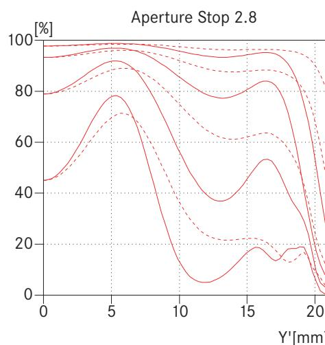
The MTF is indicated both at full aperture and at f/5.6 at long taking distances (infinity). Shown is the contrast in percentage for 5, 10, 20 and 40 lp/mm across the height of the 35 mm film format, for tangential (dotted line) and sagittal (solid line) structures, in white light. The 5 and 10 lp/mm will give an indication regarding the contrast ratio for large object structures. The 20 and 40 lp/mm records the resolution of finer and finest object structures.
