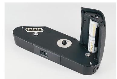
advantage that many customers have been waiting for. If the photographer does not want to use the rewind crank, he can activate the motor rewind process by means of a slide switch conveniently located for thumb operation in the centre-rear of the winder. Following this operation the film tab is left protruding
