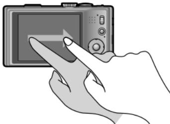
Dragging (sliding your finger across the monitor's surface) is used to scroll the pictures or change the range of the pictures displayed.
